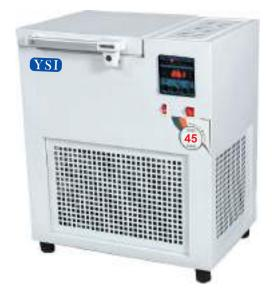
The unit serves the dual purpose i.e. it can be used as a stand alone unit, as well as, a part or subsystem of some bigger system. Temperature Range 0°C to 90°C Microprocessor based Digital Temperature Controller cum Indicator incorporating highly reliable RTD-Pt. 100 and CMOS ICs for noise immunity.
