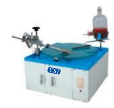
Top platform is provided with a drain to remove the used lubricant. A sector type metal scale graduated from 0 to 25° in 1° division indicates the exact angle between the bevel and center line. The unit is powder coated and complete in all respects and has aesthetic looks. Supplied with rexine cover, cord and plug without micro abrasive. Suitable to work on 220 V, single phase, 50 Hz, AC supply.
