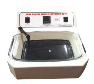
Temperature Controller fitted on the control panel. Temperature Range: Ambient to  $70^{\circ}\text{C} \pm 1^{\circ}\text{C}$  Glass Trough Size (mm):  $240(\text{L}) \times 150 \text{ (W)} \times 50 \text{ (D)}$
