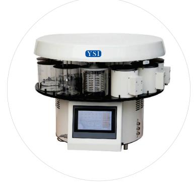
The unit is supplied complete with 2 Nos. S.S. Basket Rotors, 2 Nos. S.S. Basket, 24 Nos. S.S. Tissue Capsule, 10 Nos. S.S. beakers without lip, 2 Nos. S.S. Wax Baths (Specially designed for this model)
