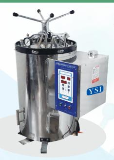
—Vertical (Digital)- Microprocessor Controlled Fully Automatic Basic Specifications are same as YSI-402 but Microprocessor Controlled. The Sterilizer Vertical is robust standing type, built, sturdy construction designed for easy operation for sterilizing culture media, glass-wares, utensils, instruments, tools etc. with steam under pressure. It is suited to
